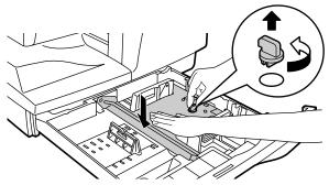
Store the pressure plate lock which has been removed in step 2 and the screw which has been removed when unpacking (see page 11, step 2 of **REMOVING PROTECTIVE PACKING MATERIALS**) in the front of the paper tray. To store the pressure plate lock, rotate the lock to fix it on the relevant location.
